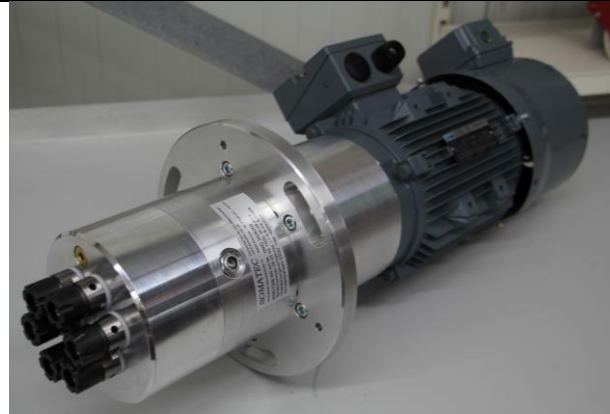
Processing unit MSK13-02 flanged to motor for drilling and tapping
