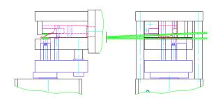
End of the cutting process; the punch can be placed in the starting position.
